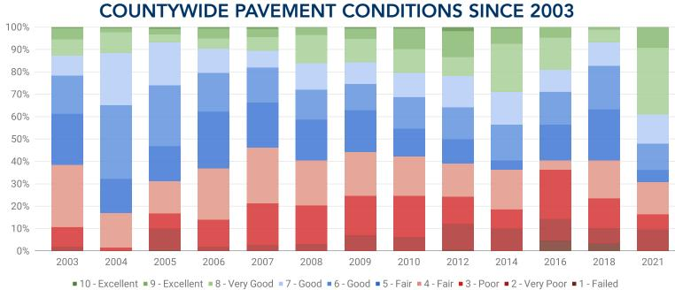
The Pavement Surface Evaluation and Rating System (PASER) is used to assign a rating from "1" (failed road) to "10" (new road/complete reconstruction). WATS, MDOT, and the WCRC have collected PASER data for Washtenaw County since 2003.
